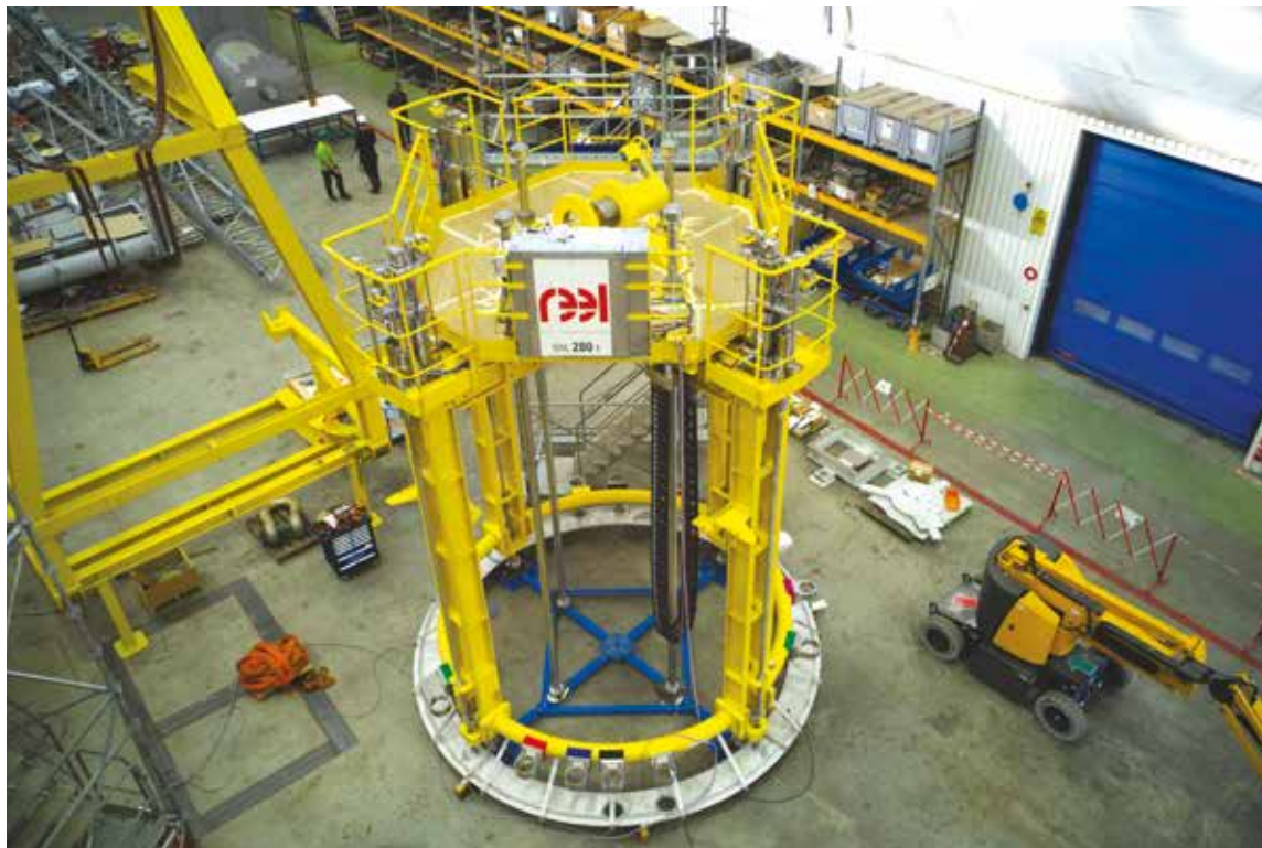
RPVI Lifting Device (OMI)
