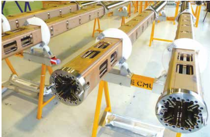
Core internals: Control Rod Guide Tubes (CRGT)
