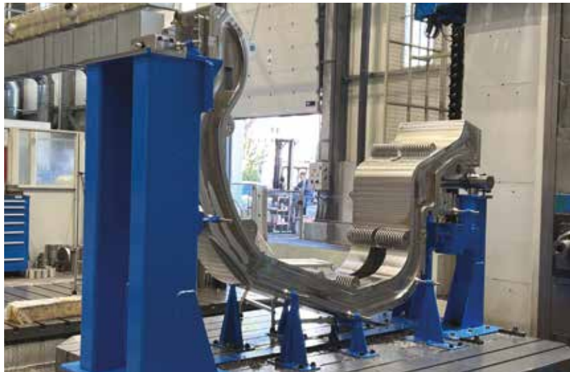
Divertor Cassettes Tokamak ITER
