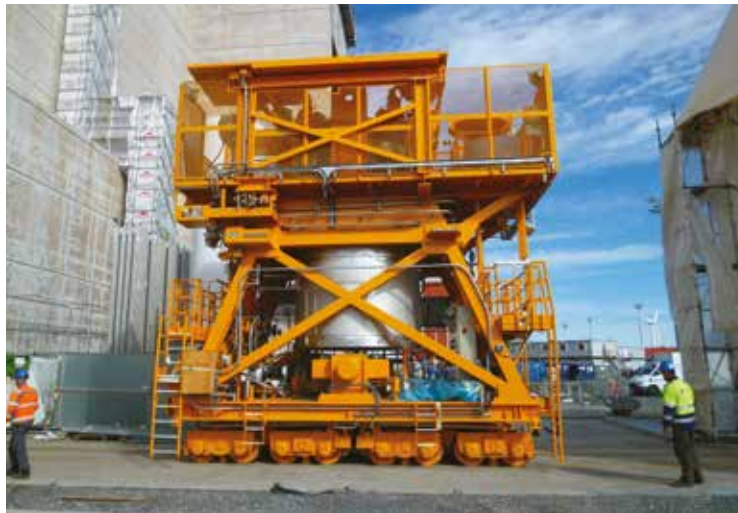
Spent Fuel Unloading System (DMK)
