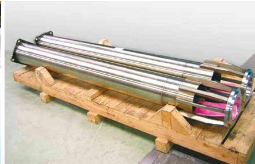
Core internals: CRGA Columns
