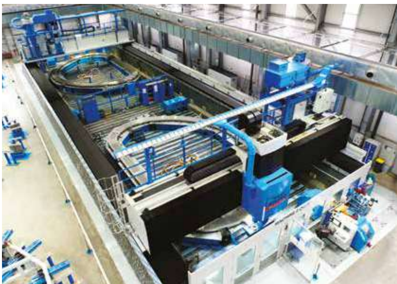
Radial plates for the ITER Tokamak being machined in the CNIM Systèmes Industriels workshops
