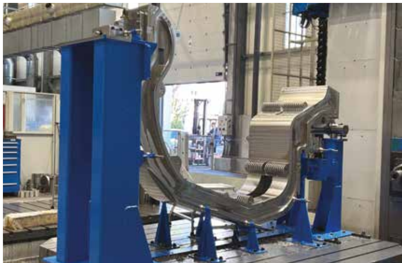
Divertor Cassettes Tokamak ITER
