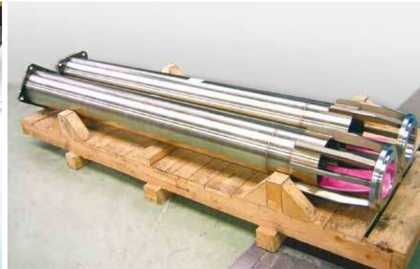
Core internals: CRGA Columns
