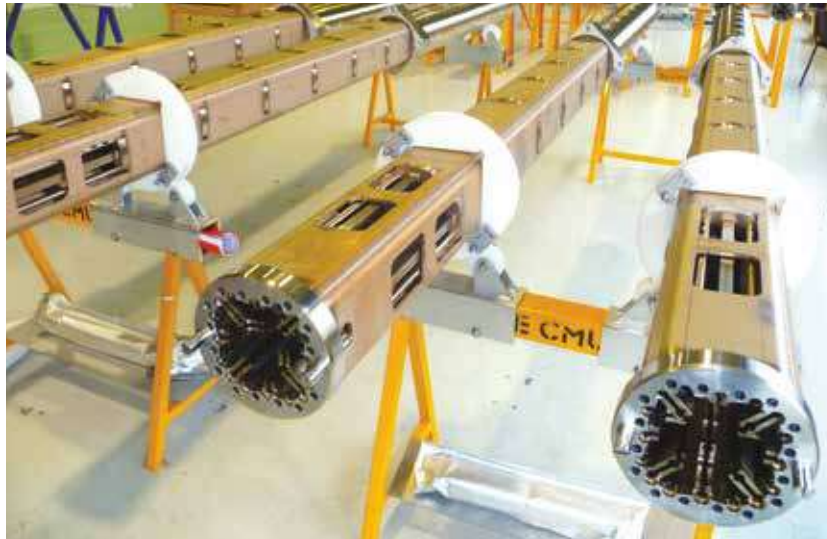
Core internals: Control Rod Guide Tubes (CRGT)
